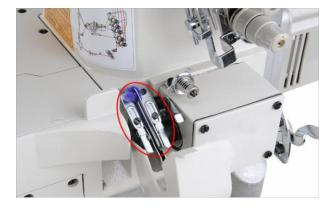
**3**. Cam anti-wrap, far away from tangled lines Cam anti-wrap:prevent the bottom thread wrap on the thread cam after breaking, improving production efficiency;Quick positioning: thread cam is easy to
